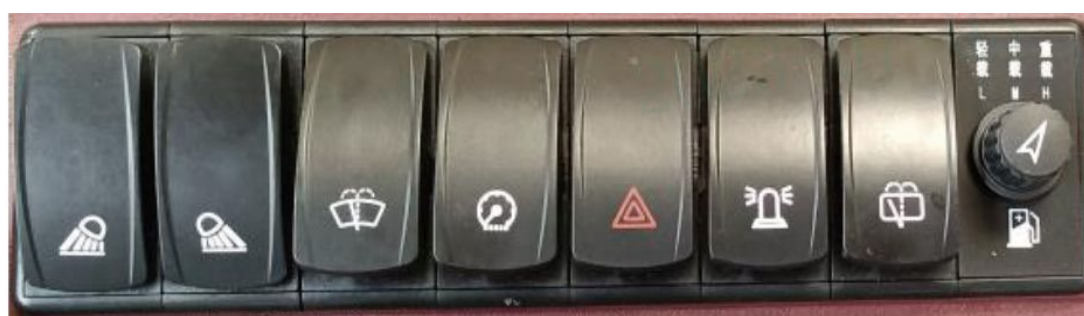
Rocker switch assembly (on the right door trim panel)
